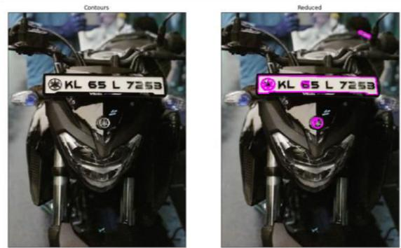
By the modified version of the Connected Component Analysis py script concept, other fields that may not be license plates have been exhausted. Finally, we get number plate.
